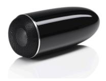
**Aluminium tweeter** CM10's tweeter is of a sandwich construction. The visible dome is attached to a second layer that replicates the main dome's profile with the centre cut out. This raises the first break-up frequency to 38kHz, for more pistonic behaviour in the audible range.
