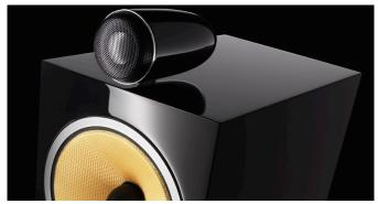
**Tweeter on top** For the first time in the CM Series, the tweeter is mounted in its own dedicated housing on top of the cabinet, which improves high-frequency dispersion, aids imaging and endows the CM10 with a more "out of the box" sound than its conventional siblings.
