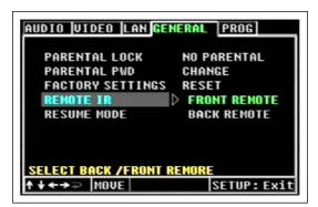
**Note:** After changing this option you will not be able to use the remote control to control the DVD26. You can reset this option to the front remote setting by switching off the power, using the power switch under the left-hend edge of the front panel.
