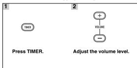
Each time you press **TIMER** while the power is on, it switches on/off. When you switch on the timer, the TIMER indicator lights up on the front panel display ( $\mathbb{F}$  P. 6). To turn on the unit via the timer, set this unit to standby mode when the timer is switched on.
