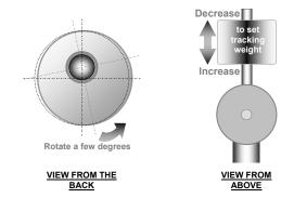
Hold the bearing yoke and with a gentle rocking motion push it down. The bearing will disengage from its locked transit position and the unipivot spike screw will fall into its bearing seat ready for normal use. Now remove the beaded tie-wrap to release the arm.
