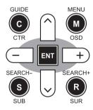
**MENU/OSD button:** Press to display the SYSTEM STATUS screen. From the SYSTEM STATUS screen, press the ENTER button to display the MAIN MENU screen which has links to all other menus. If a menu is already visible, push this button to cancel the display. The MENU button on the front panel provides the same function.
