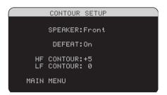
The CONTOUR SETUP menu allows digital adjustment of the bass and treble response of each group of speakers in the system. For example, if your center channel speaker sounds too bright, you could roll off the extreme high frequencies.
