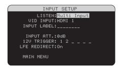
When the MULTI INPUT source is selected on the INPUT SETUP menu, the available options change to reflect the fact that these inputs are direct analog inputs and bypass the receiver's digital processing. The INPUT, CINEMA EQ, DEFAULT MODE and GROUP DELAY options are not available since these are all digitally implemented features.
