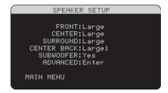
The SPEAKER SETUP menu is used to configure the receiver for use with your specific loudspeakers and to determine the bass management configuration as described in the previous overview. The menu is accessed from the MAIN menu.
