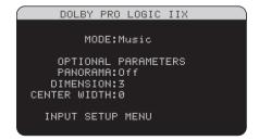
When Dolby Pro Logic IIx is selected as the default surround mode on the INPUT SETUP menu, there are additional settings and parameters to optimize the surround decoding for music or movie soundtracks. Dolby Pro Logic II uses matrix decoding algorithms to derive a center channel and surround channels from 2-channel source material.
