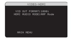
The VIDEO/HDMI menu deals with the configuration of the HDMI and Component output for high-definition video display devices. See the Video Inputs & Outputs section of this manual.
