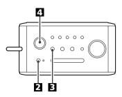
Connect the PHONES jack (audio output jack) of a portable audio player to the AUX IN jack of the R-3 using the supplied stereo mini plug cable.
