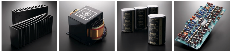
Large heat sink, huge power transformer, custom-made block capacitors (24,000µF) and preamp board.
