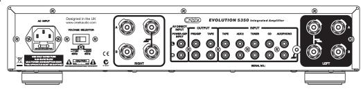
The rear panel, from left to right, features a mains inlet socket with fuse and voltage selector switch. Right channel A and B speaker output terminals. AV Direct or Power amp Input, Pre-amp and tape outputs. Tape, Aux 2, Tuner, CD and Aux or Phono Inputs. Ground post. Left channel speaker A and B output terminals.
