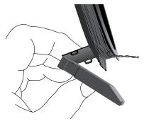
2. Push the tab into the open slot in the base of the stand. Press until the tab clicks home.
