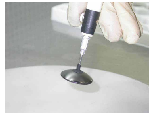
A Perfect Mix: An USHER Diamond DMD dome has a proprietary metal alloy base layer coated with an amorphous diamond-like carbon layer on both sides. Pure diamond is carbon atoms arranged solely in sp^3 bonds; amorphous diamond-like carbon has mixed sp^3 and sp^2 bonds to achieve its desirable properties
